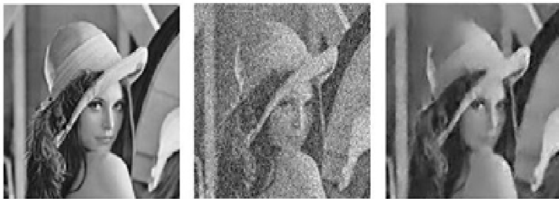
FIGURE 2: From left to right: original image, noisy image with zero-mean white Gaussian noise of \|n\|_2 = 20 , the cleaned image via ICA based sparse representation described.
