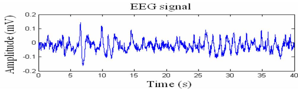
**FIGURE 1:** EEG Signal corrupted with ECG/EKG and line signals (*adapted from Artifact Removal from EEG Signals using Adaptive Filters In Cascade, A Garcés Correa et al, Journal of Physics: Conference Series 90, 2007*)
