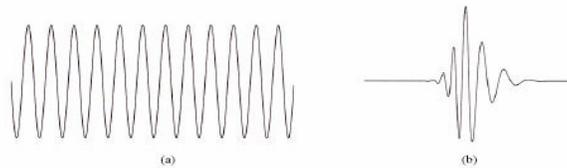
**FIGURE 2:** Demonstration of (a) a wave and (b) a wavelet. Notice that the wave has an easily discernible frequency while the wavelet has a *pseudo frequency* in that the frequency varies slightly over the length of the wavelet. (adapted from D.L. Fugal. 2009. *Conceptual Wavelets in Digital Signal Processing: An in depth Practical Approach for the Non-Mathematician*, Space & Signals Technologies LLC)
