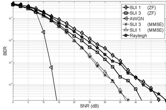
FIGURE 3: Performance Simulation (ZF and MMSE)
