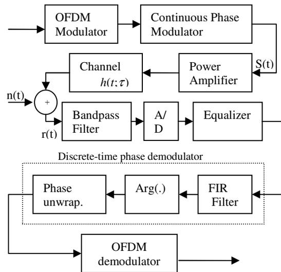
FIGURE 1: OFDM-CPM block diagram.
