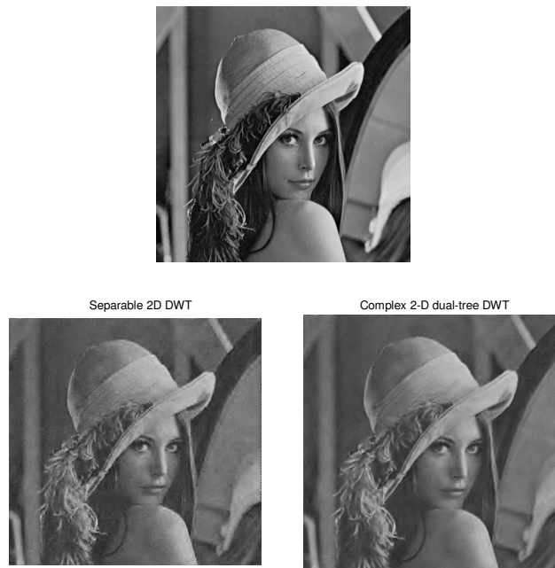
Figure 5: (a) Input Image, (b) Denoised with real CWT,(c) Denoised with dual tree CWT
