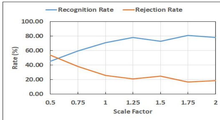
FIGURE 10: Effect of image scale on recognition and rejection rates.
