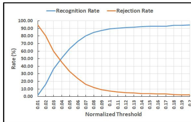
FIGURE 8: Effect of distance threshold on recognition and rejection rates.
