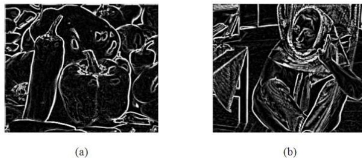
FIGURE 17: Enhanced edges after applying top-hat transform (3x3 SE); (a) Pepper (b) Barbara.
