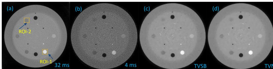
**FIGURE 3:** (a) Scanned CATPHAN image with the scanning parameters of 100 kV<sub>p</sub>, 20 mA and 32 ms (used as a “Gold Standard” image), (b): Same CATPHAN scanned with 4 ms (used as a low-dose noisy image), (c) and (d) Processed 4 ms CATPHAN image through TVSB and TVN algorithm respectively. Regions of interest (ROIs) for computing the CNRs were shown in Fig. 3(a).
