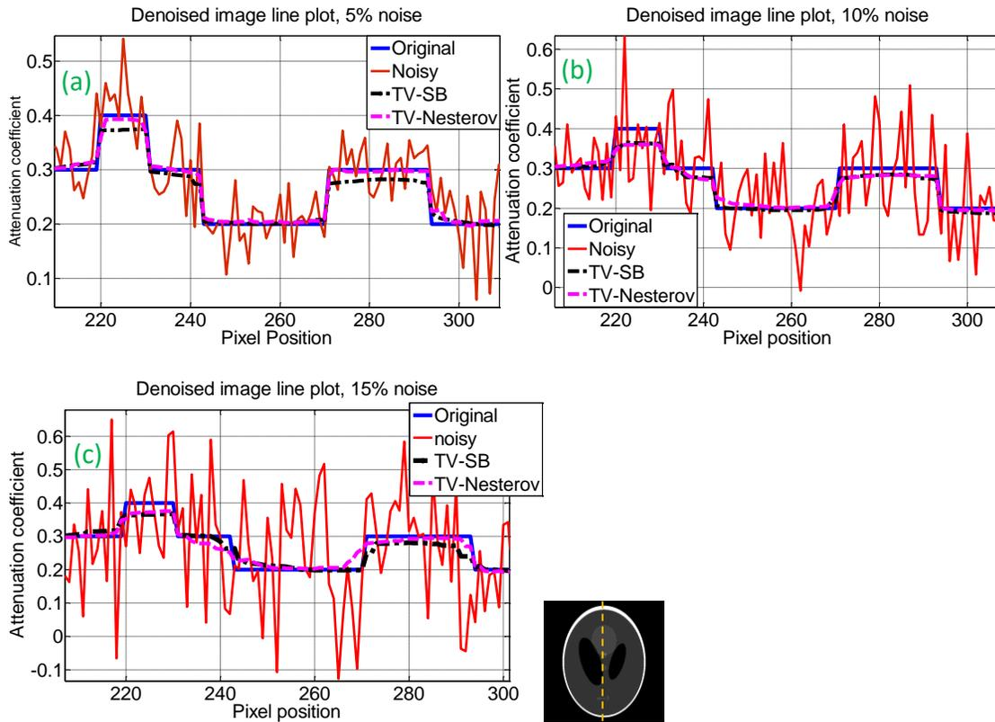
**FIGURE 2:** (a) , (b) and (c): Line profiles of original, noisy and denoised Shepp-Logan phantom for 5%, 10% and 15% Gaussian noise respectively. The line profile was plotted across the dashed yellow vertical line shown on the phantom image.
