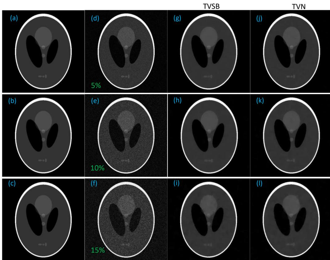
**FIGURE 1:** (a) ,(b) and (c) Original 512 x 512 Shepp-Logan Phantom, (d) ,(e) and (f) 5%, 10% and 15% additive Gaussian noise added to the phantom respectively, (g) ,(h) and (i) Respective denoised images using TVSB, (j),(k), and (l) Respective denoised images using TVN.
