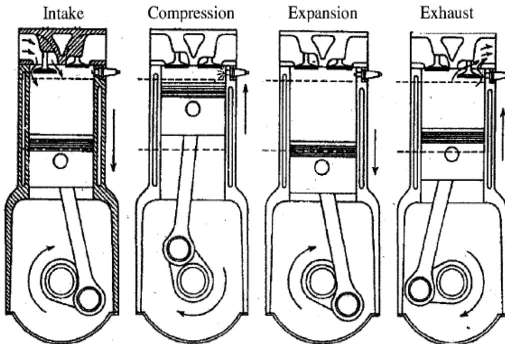
FIGURE 1: The Four Stroke Engine Cycle [1]
