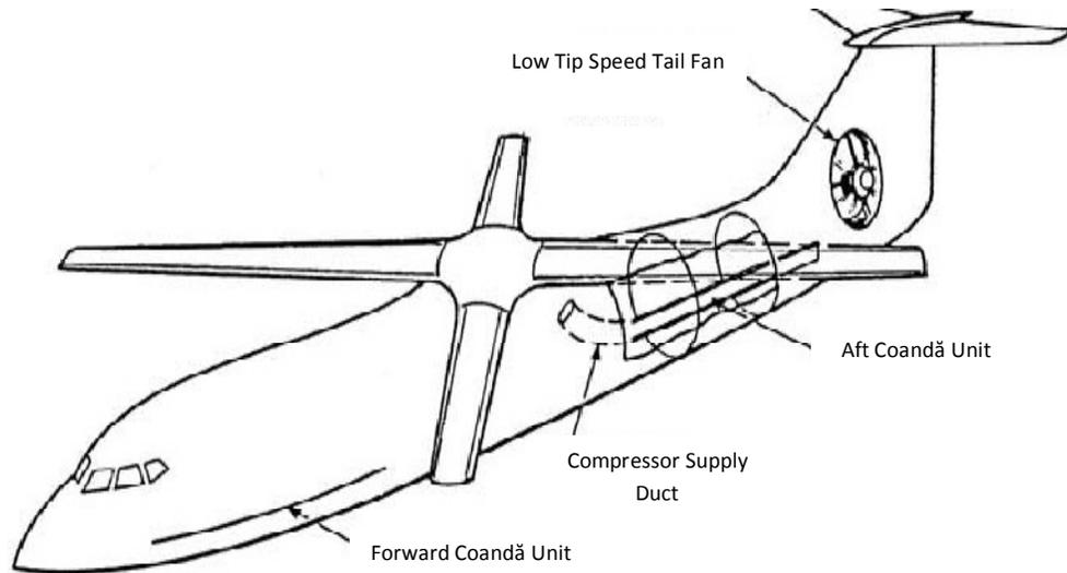
**FIGURE 5.** X-Wing Configuration and Supply Compressor.
