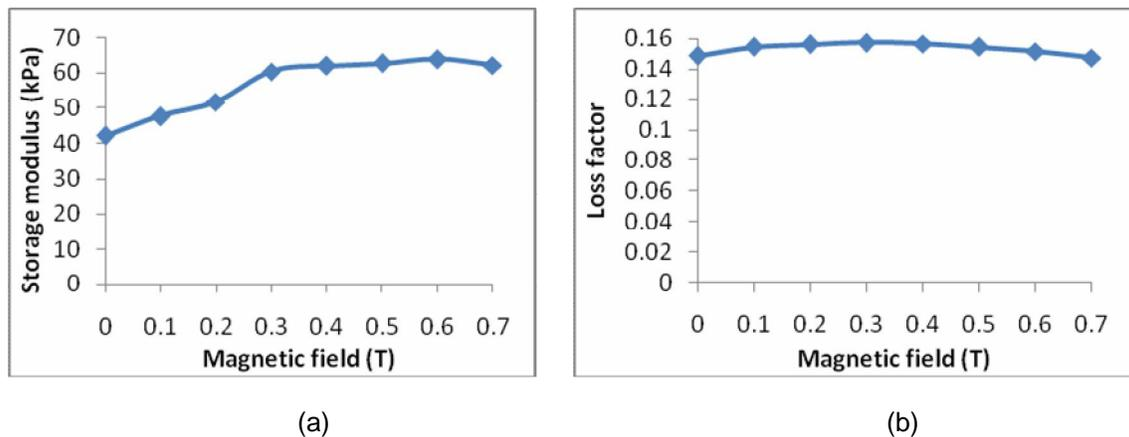
**FIGURE 8:** (a) Storage modulus, and (b) loss factor of the gel with 50% by weight of carbonyl iron particles under different magnitudes of magnetic field.
