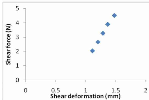
**FIGURE 6:** Static shear force vs shear deformation of magnetic composite gel with 50% by wt. of carbonyl iron particles at 0.7 T magnetic field.
