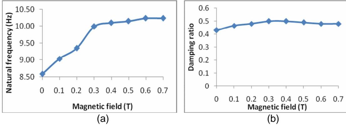
**FIGURE 7:** The response of the system measured in terms of (a) *natural frequency* and (b) *damping ratio* with a gel (consists of 50% by weight of carbonyl iron particles) mounted under varying magnetic field.
