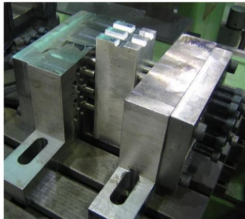
**FIGURE 1:** Prototype of Pin Type fixture
