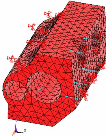
**FIGURE 5:** Sample workpiece evaluated using FEA for final clamp configuration
