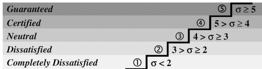
FIGURE 9: The quality maturity levels and their scales for the Software Product Quality Maturity Model (SPQMM) (Al-Qutaish & Abran, 2011).
