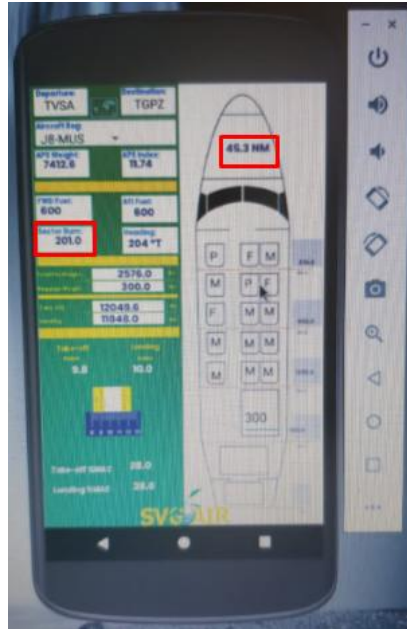
FIGURE 4: Sector Burn for the flight in pounds as well as the distance in Nautical Miles.
