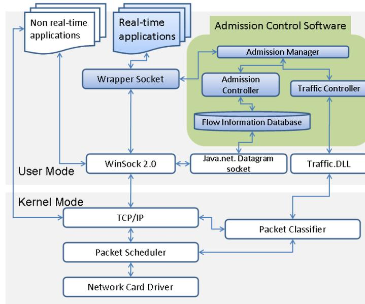
FIGURE 10: Windows Based soft real-time system Architecture.
