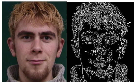
FIGURE 6: Illustrates the edge detection algorithm (Canny): (a) original image (b) resulting image
