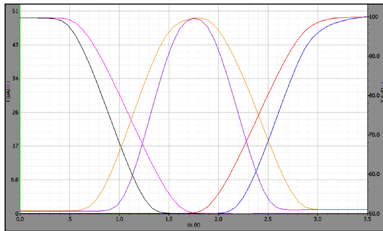
FIGURE 18: UMFs and LMFs of 3 FOUs for one variable obtained through simulation of fuzzifier circuit W/L=4 for UMFs, 3 for LMFs
