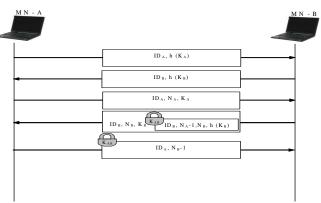
FIGURE 2: Secure Route Data Communication between Mobile Node A and Mobile Node B
