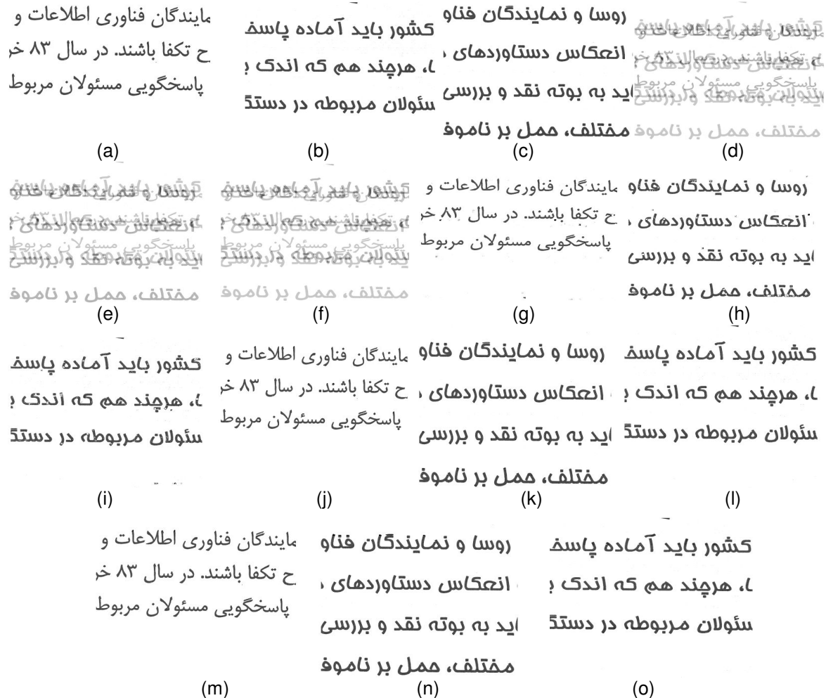
FIGURE 3: a, b, c) original sources. d, e, f) three synthetic mixtures in noiseless system. g, h, i) reconstructed sources using BSS by 4*4 mosaic size. j, k, l) reconstructed sources using BSS by 16*16 mosaic size. m, n, o) reconstructed sources using BSS by 64*64 mosaic size.
