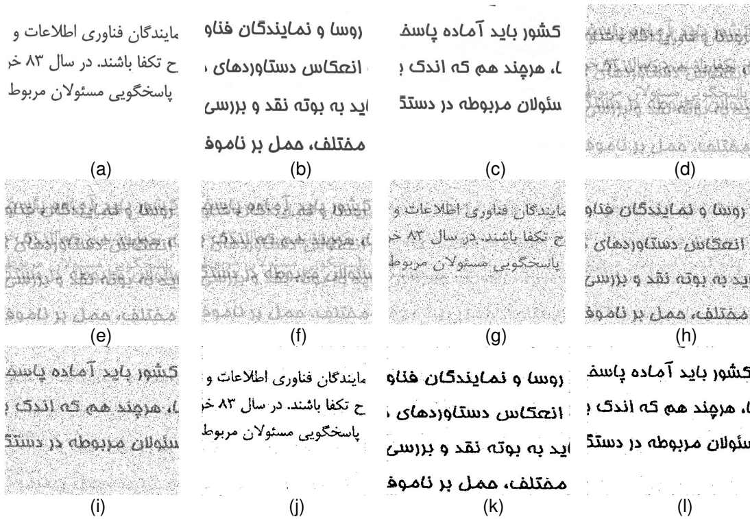
Figure 10: a, b, c) original sources. d, e, f) 3 mixtures added 10% salt & pepper noise. g, h, i) reconstructed sources using proposed algorithm. J, k, l) enhancement of the results using binarization method.
