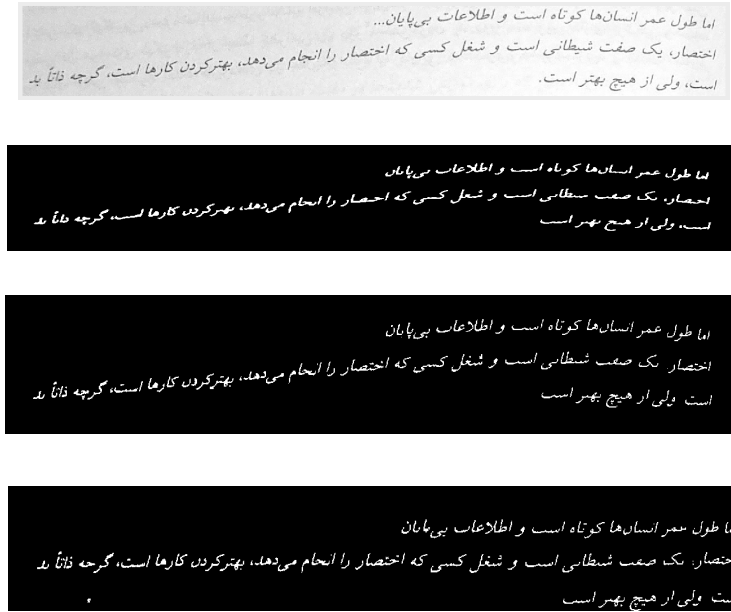
FIGURE 5: from top to down – a. the original image, b. elimination of the noisy areas, determination of the boxes and the text lines, c. estimation and correction of the skews of the boxes, d. transformation of the boxes and the output image of the algorithm.
