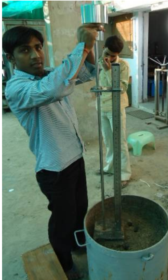
FIGURE 5: Dynamic Cone Penetrometer
