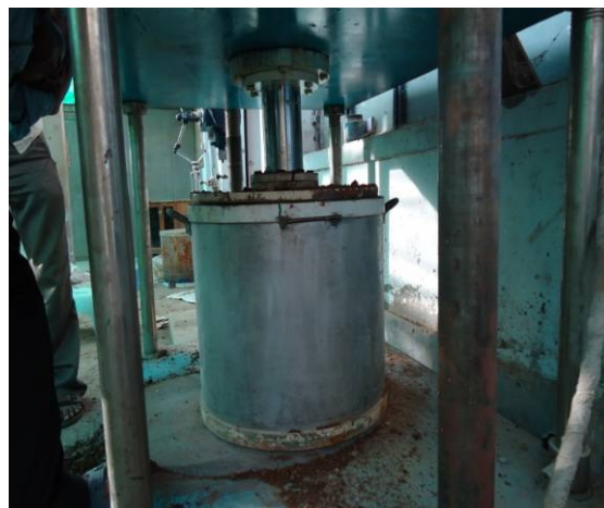
FIGURE 4: Compression testing machine for static Compression of sample in mould
