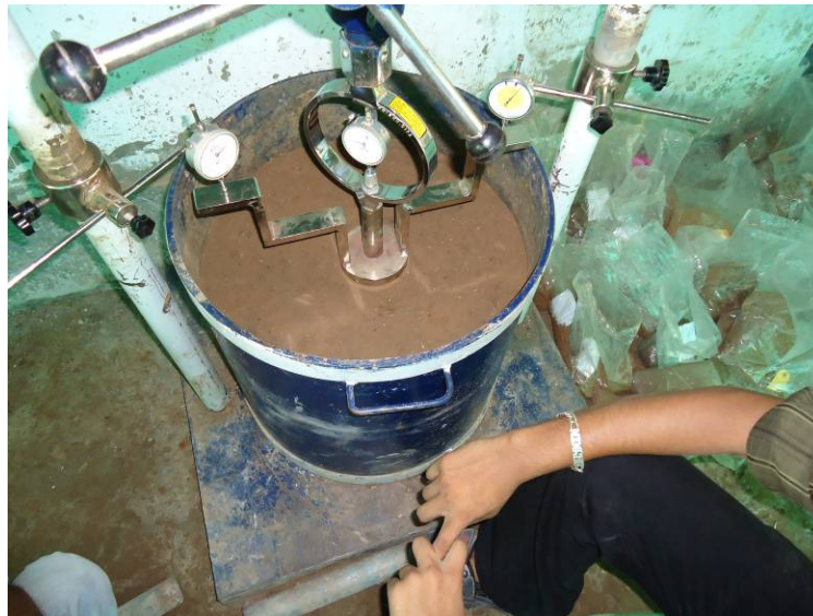
FIGURE 2: The photograph of mould and Reaction frame
