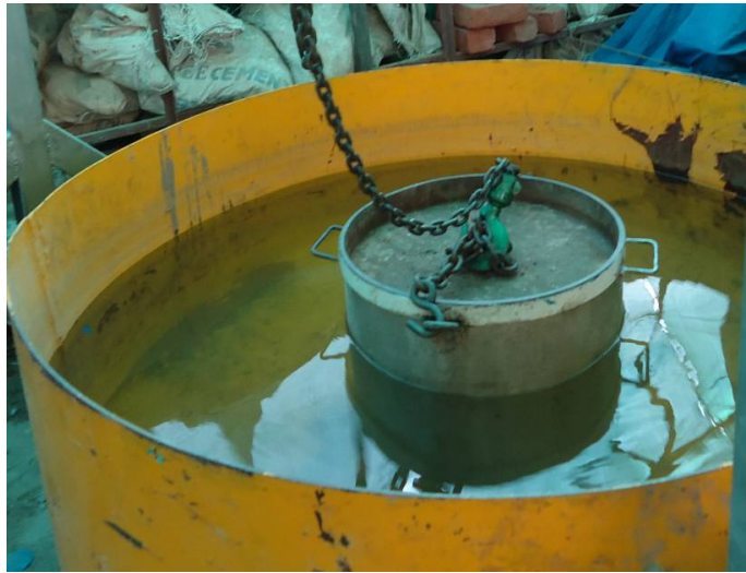
FIGURE 3: Mould with saturation tank
