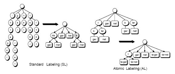
FIGURE 5: Labeling each Node with a Syllable Instead of a Single Character
