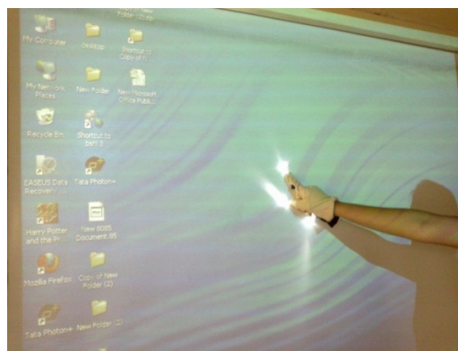
Figure 4: Mouse Cursor tracking with single LED
