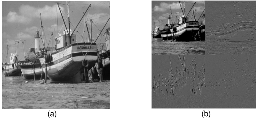
FIGURE 4: (a) Original image of boat, (b) Result after the one-level 2-D Haar-DWT
