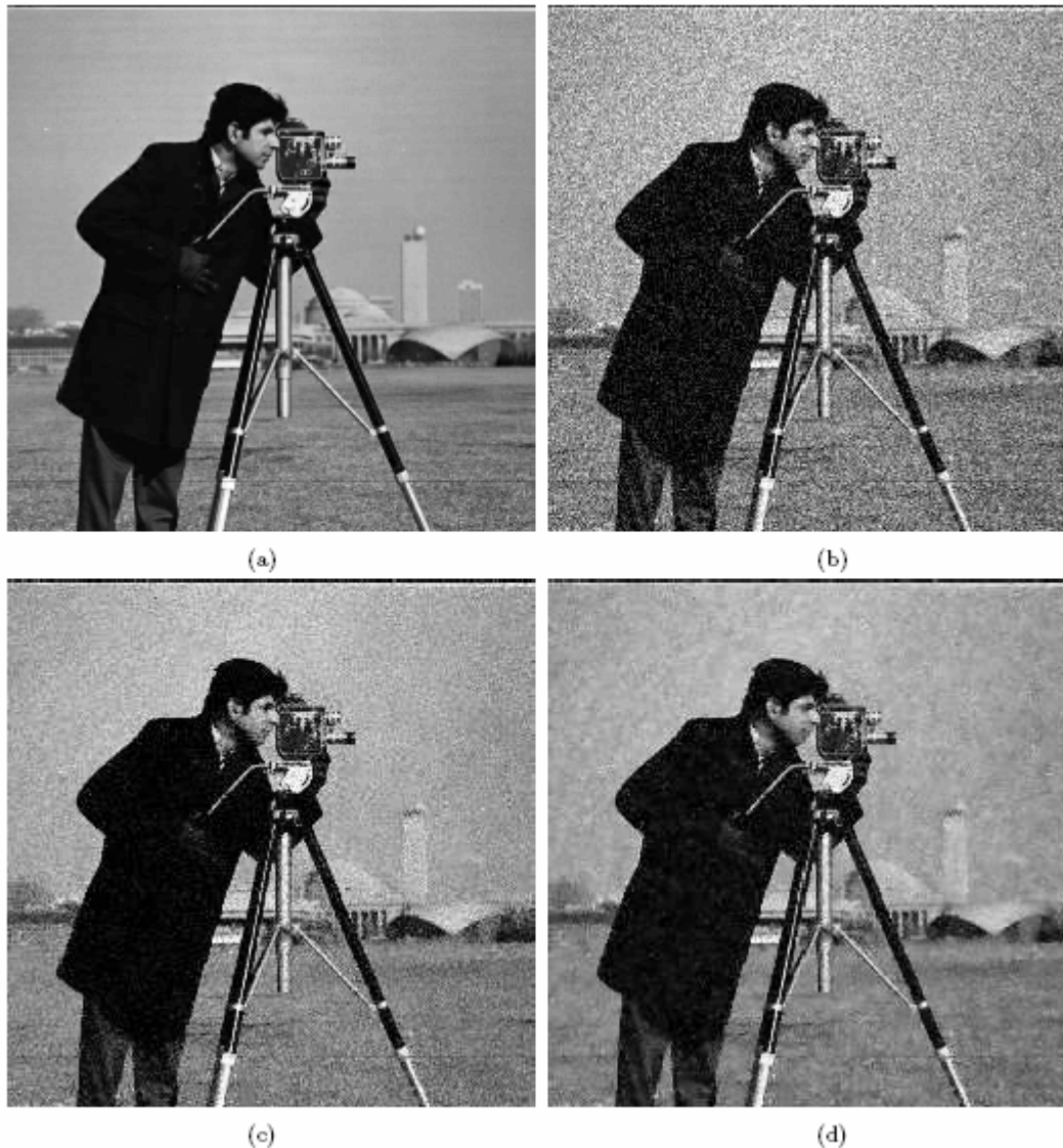
Figure 4: Cameraman test image: (a) Original image. (b) Noisy image (PSNR = 20.65). (c) Bilateral filtering (PSNR = 24.70). (d) The proposed method (PSNR = 26.00).
