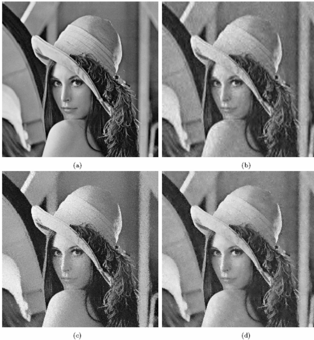
Figure 6: Lena test image: (a) Original image. (b) Bayesshrink (PSNR = 29.06). (c) Bilateral filtering (PSNR = 28.70). (d) The proposed method (PSNR = 30.09).
