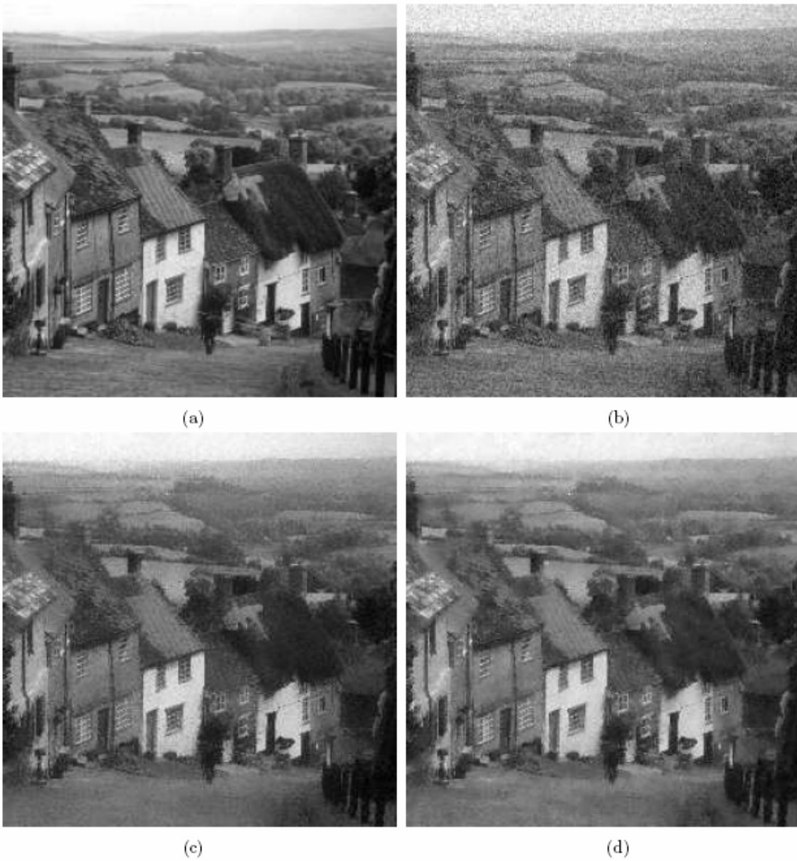
Figure 5: Goldhill test image: (a) Original image. (b) Noisy image (PSNR = 24.71). (c) Bilateral filtering (PSNR = 27.81). (d) The proposed method (PSNR = 28.56).
