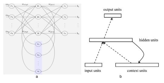
FIGURE 6: Elman recurrent network. (a) From [16] (b) from [18].
