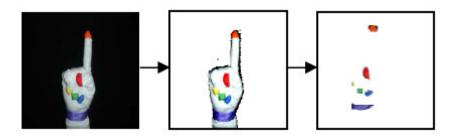
FIGURE 8: Color segmentation using colored glove [26].
