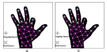
FIGURE 13: (a) False finger detection, (b) correct finger detection, by applying the mean finger length comparison check [28].
