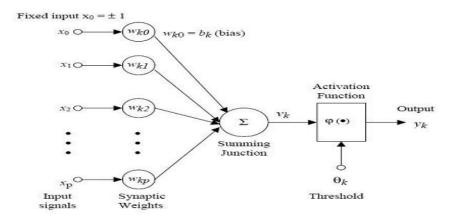
FIGURE 3: Representation of simple artificial neuron (From internet image gallery).
