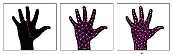
abCFIGURE 12: Growth of the SGONG network: (a) starting point 2 neurons, (b) growing stage 45 neurons and (c) final<br/>output grid of 83 neurons [28].
