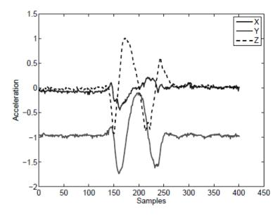
FIGURE 10: Acceleration signals was recording when the hand performing a circular motion [31].
